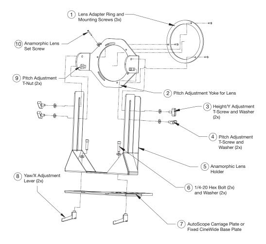
Figure 3-17. Cylindrical Anamorphic Lens Mounting Assembly - Exploded View
